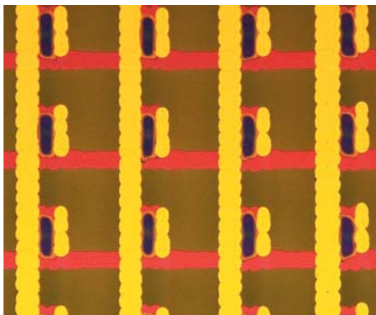
PLASTIC TRANSISTOR ARRAYS were patterned using ink-jet printing by the Palo Alto Research Center (PARC). The lower image shows 12 transistors of an array. The dots are about 40 microns in diameter. The researchers used a semiconducting polymer ink developed by Beng Ong of the Xerox Research Center of Canada. The transistors would be suitable for use in active-matrix displays, electronic paper and other applications.
